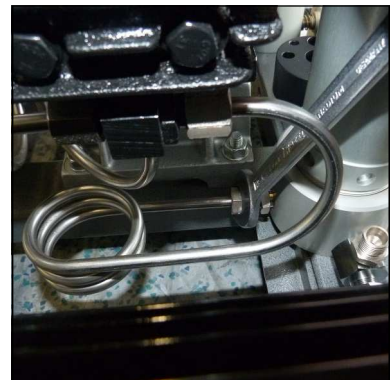
Fig. 2 - Loosen pipe connections of the filter housing
