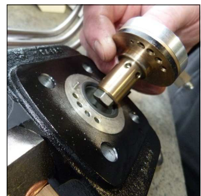
Fig. 5 - Ensure correct valve position (centre pin)
