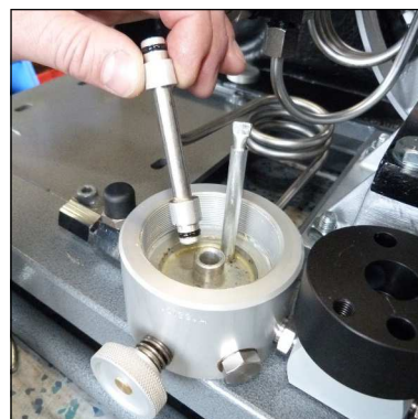
Abb. 5 - Remove duct collar and change o-rings
