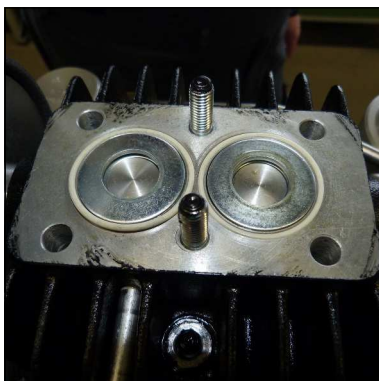
Fig. 5 - Spring plate inside the valve head
