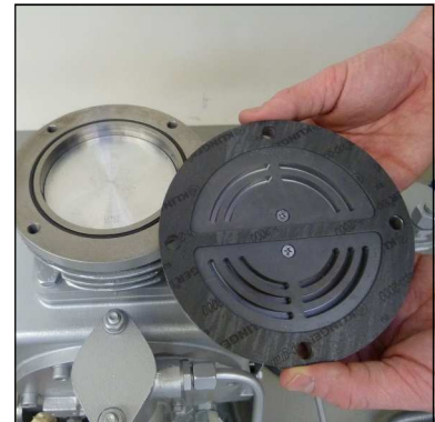
Fig. 2 - Correct mounting position of upper valve gasket
