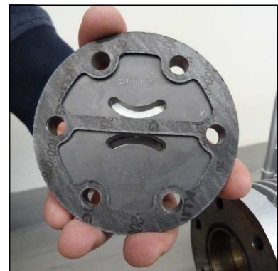
Fig. 2 - Correct mounting position of upper valve gasket
