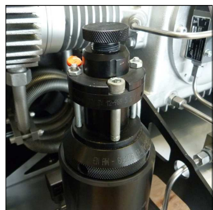
Fig. - Safety valve 3rd stage
