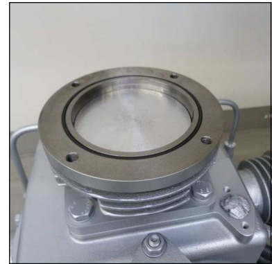
Fig. 1 - Change lower gasket (o-ring)
