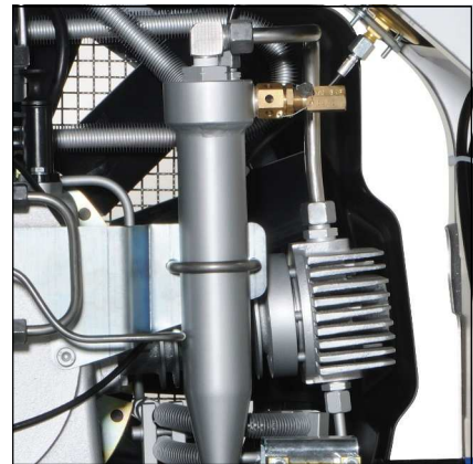
Fig. 1 - Oil / water separators after 2nd stage with automatic condensate drain system
