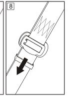
Adjusting the thigh straps and work positioning belt
