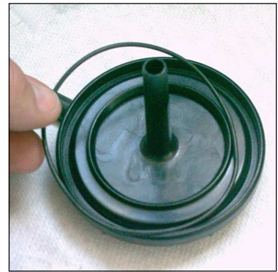
Fig. 3 - Place o-ring into the filter housing
