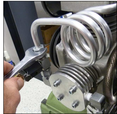
Fig. 1 - Loosen pipe connections
