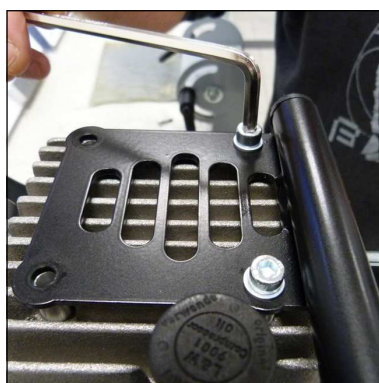
Fig. 3 - Loosen valve head screws
