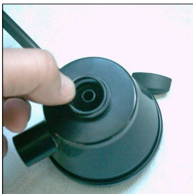
Fig. 4 - Place o-ring into the groove
