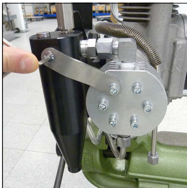
Fig. 1 - Loosen mounting screws
