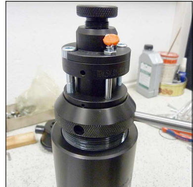
Fig. 1 - Remove/screw in filter cover
