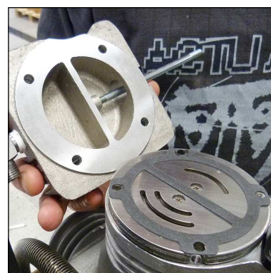
Fig. 4 - Remove valve head
