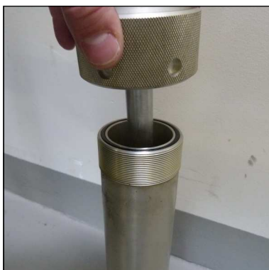
Abb. 4 - Remove lock ring and change o-ring
