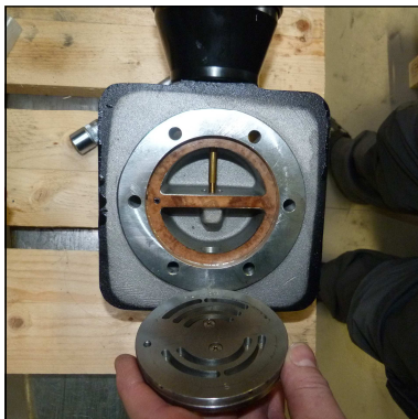
Fig. 2 - Correct position of in-and outlet valve
