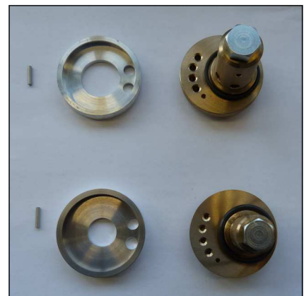
Fig. 2 - In - and outlet valve c/w gaskets 2nd stage (top) und 3. Stufe (below)
