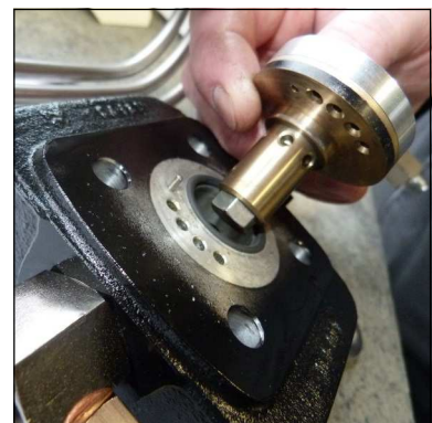
Fig. 4 - Ensure correct valve position (centre pin)
