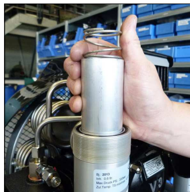
Abb. 2 - Remove filter cartridge
