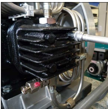
Fig. 2 - Loosen valve head screws
