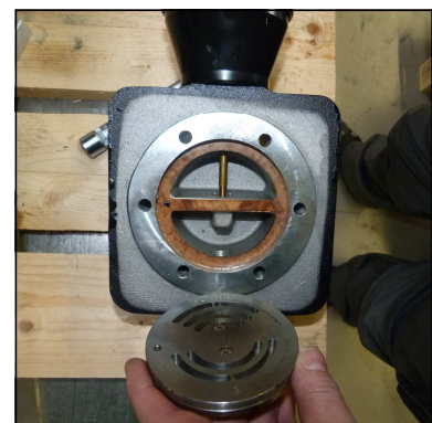
Fig. 5 - Remove in- and outlet valve
