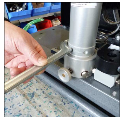
Abb. 3 - Turn off filter housing
