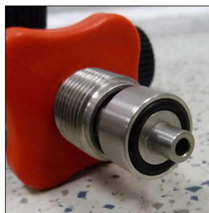
Fig. 1 - O-ring at the filling valve
