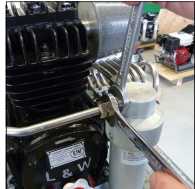
Fig. 1 - Loosen pipe connections of the water separator
