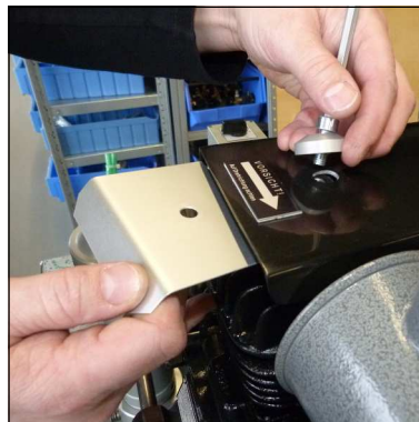
Fig. 2 - Remove protection plate
