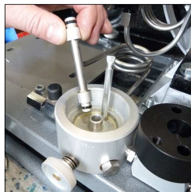
Abb. 5 - Remove duct collar and change o-rings
