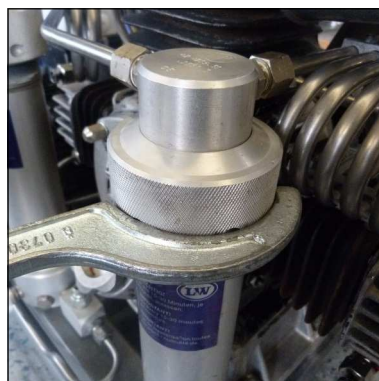
Abb. 5 - Tighten lock ring
