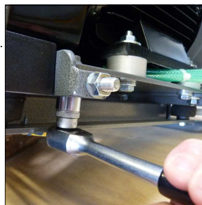
Fig. 1 - Loosen mounting screws of the motor flange
