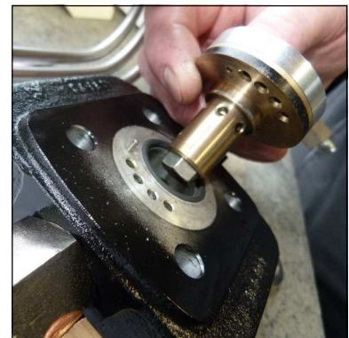
Fig. 5 - Ensure correct valve position (centre pin)
