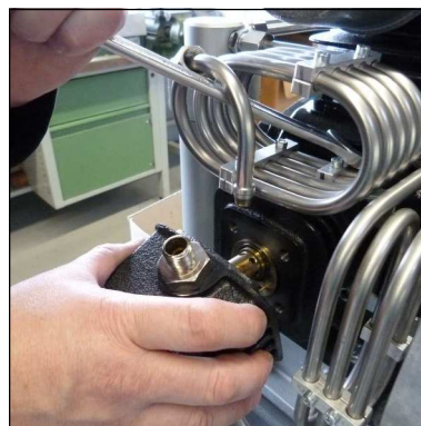
Fig. 3 - Remove valve head
