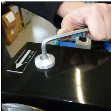
Fig. 1 - Remove top mounting screws
