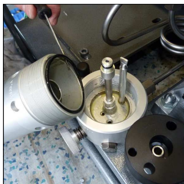
Abb. 4 - Remove lock ring
